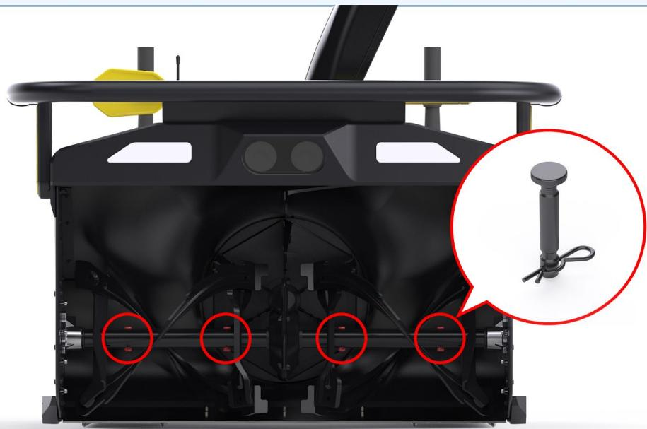
**Q Auger NOT spinning?    A Check the Shear Pin.**
